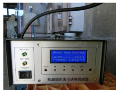
Testing device for disconnection point
