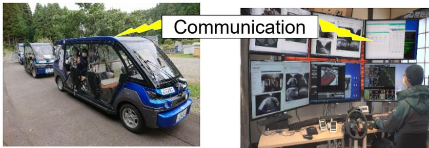
One remote-monitoring operator controls three unmanned automated driving cars.
