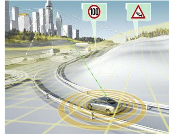
V2X via location-cast is about Electronic Horizon far ahead of the vehicle:
