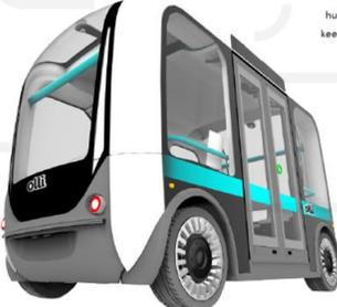
**SENSITIVE:** My lidar and optical cameras allow me to see in all directions.
