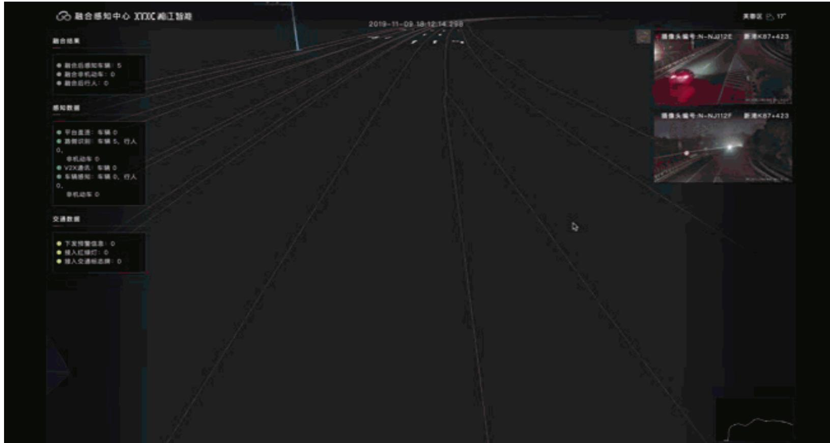
**Cooperative Perception:** Roadside camera and radar to sense the real-time status of traffic (the direction of the speed of pedestrians, motor vehicles, and non-motor vehicles), combined with high-precision maps, sent to vehicles
