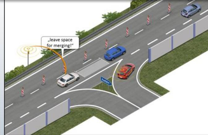
Infra suggest info to coordinate right of way in a way to optimise the overall traffic flow
