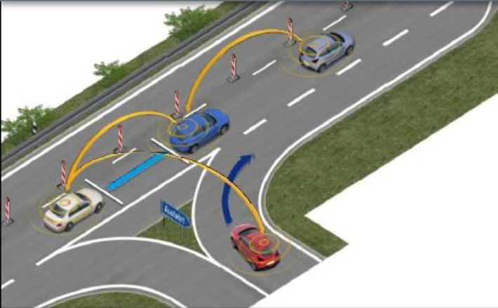
Based on notification of intended merging, interested vehicles exchange info to coordinate gap opening and merging maneuvers with increased time spans
