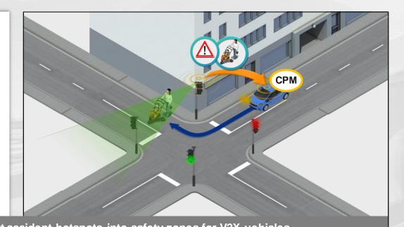
Smart Intersections with CPM can convert accident hotspots into safety zones for V2X vehicles Smart intersection & CPM sending vehicles are the only available technology to protect VRU in NLOS situations
