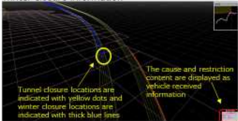
Highway (1) tunnel closure information and winter closure information
