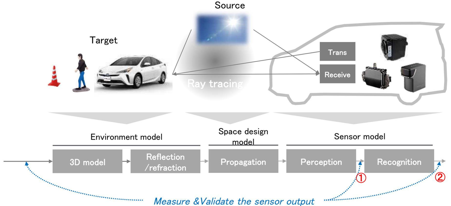
**Measurable or not is also the key feature for sensing limit definition**
