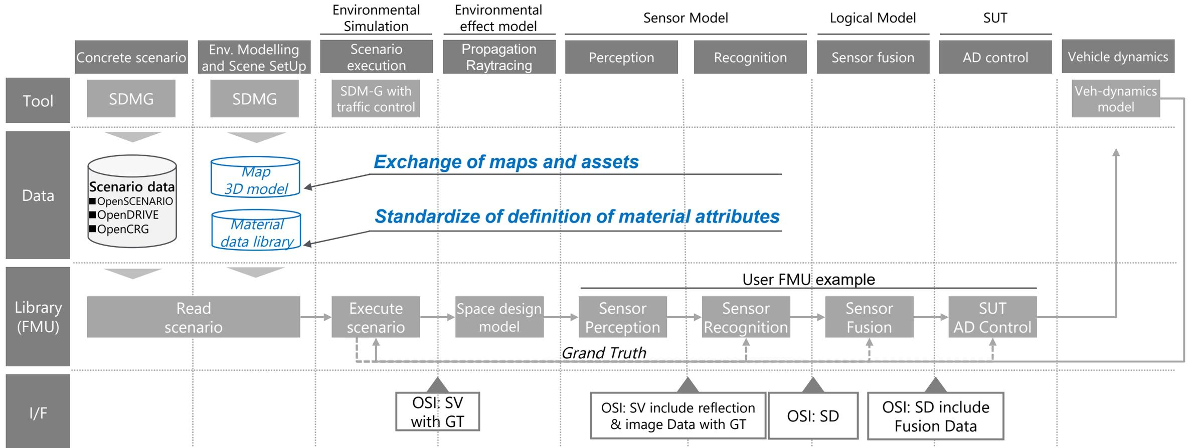
Note SDM-G: Space Design Model Generator, SV: Sensor View, SD: Sensor Data, GT: Grand Truth
