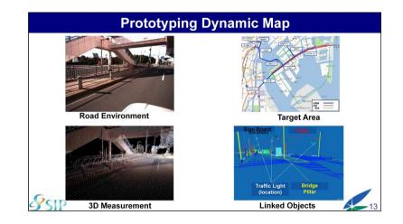
We developed a prototype of basic map layer in the target area of early deployment, Tokyo bay area.
