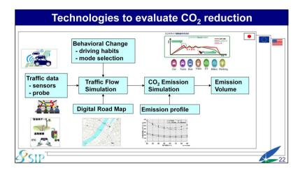
With traffic information from fixed sensors and moving vehicles combined, and detailed digital road map, we can precisely reproduce movement of each vehicle on the computer.
