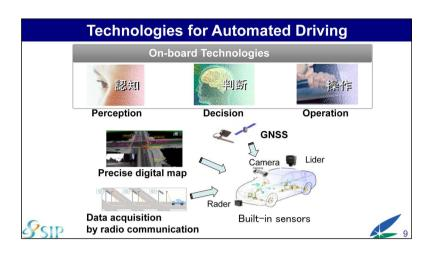
Automated driving will be realized integrating on-board technologies, precise digital map, data acquisition through radio communication and global positioning.
