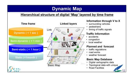
We are searching for structure of dynamic map built on shared map database. We are discussing layers with different time frame; static, semi-static, semi-dynamic and dynamic.
