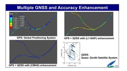
We collected data while driving a car with monitoring equipment.
